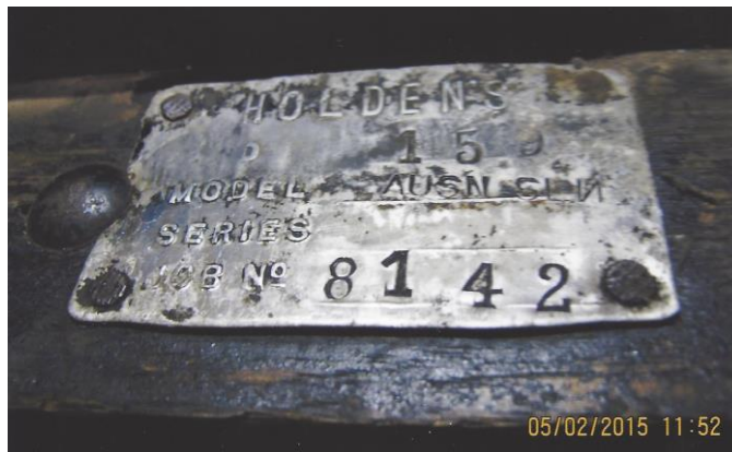
Original HOLDEN'S aluminium body plate under the back seat, stamped BODY No 159, MODEL AUSN SLN, JOB No 8142.
