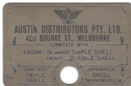
This Austin Distributors plate is bolted to the off side fuel tank bolt
