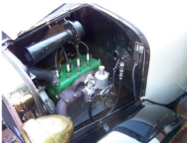
The Chummy after fitting a 1928 coil engine and 1 1/8" SU
